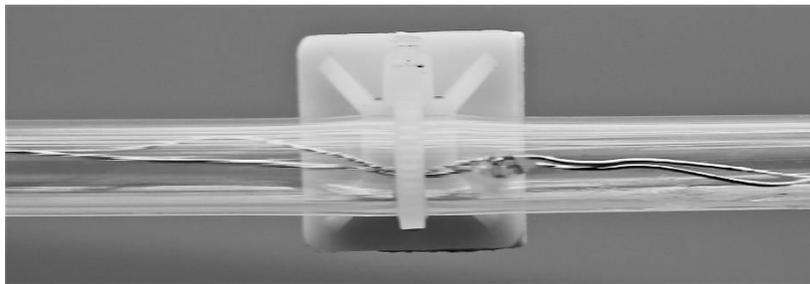
Install **backboard string light** by “outlining” backboard with light string (longer of 2 strings). Secure with zip ties at each fastener.
