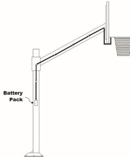
**Step 6 - Attach Battery Pack** to basketball pole. *Recommended location:* on the back or side of pole. Remove adhesive covering and press firmly to attach to pole.
